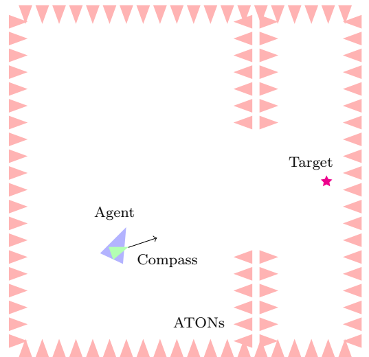
Fig. 4: Illustration of ghost boids. ATONs (red triangles) point away from danger for collision avoidance. A compass (green) is located on an informed agent (blue) and points toward the target (magenta) for goal-seeking behavior.
