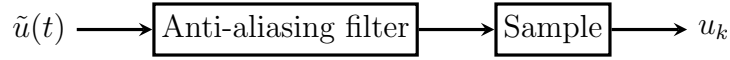
Figure 2.1. Obtaining a discrete-time signal from a continuous-time signal. The continuous-time signal \tilde{u}(t) is passed through an anti-aliasing filter and sampled to obtain a discrete-time signal u_k .
